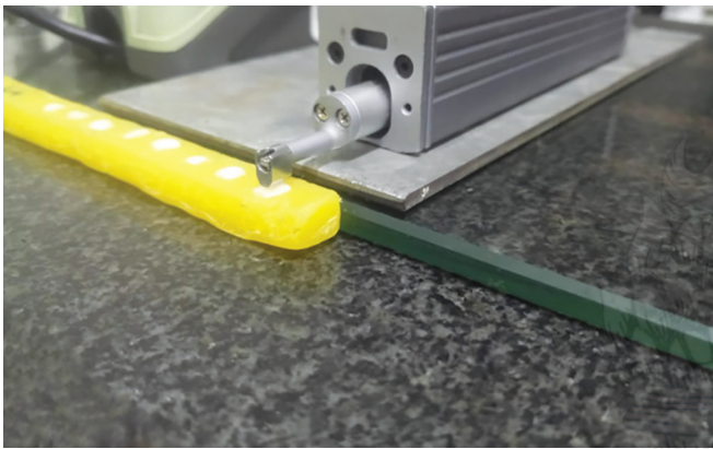
Fig. 5: Measurement of the microroughness of the dental surface
