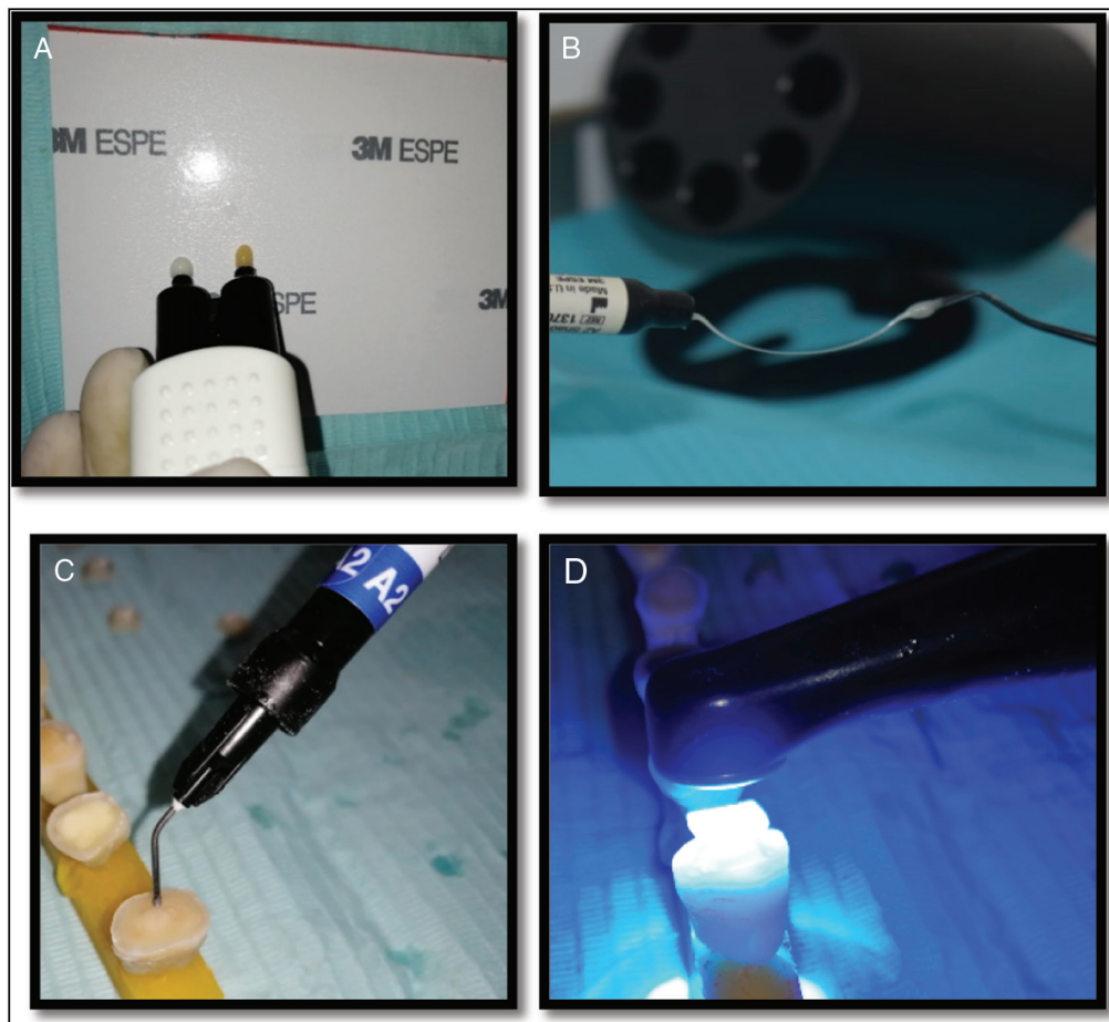
Figure 2: A: Dual RelyX™U200 Self-Adhesive Resin Cement Preparation. B: Z250XT resin composite preheating. C: Placement of Z350XT Flowable resin composite. D: Light curing of samples with third generation LED curing lamp (Valo - Ultradent, South Jordan, UT, USA)
