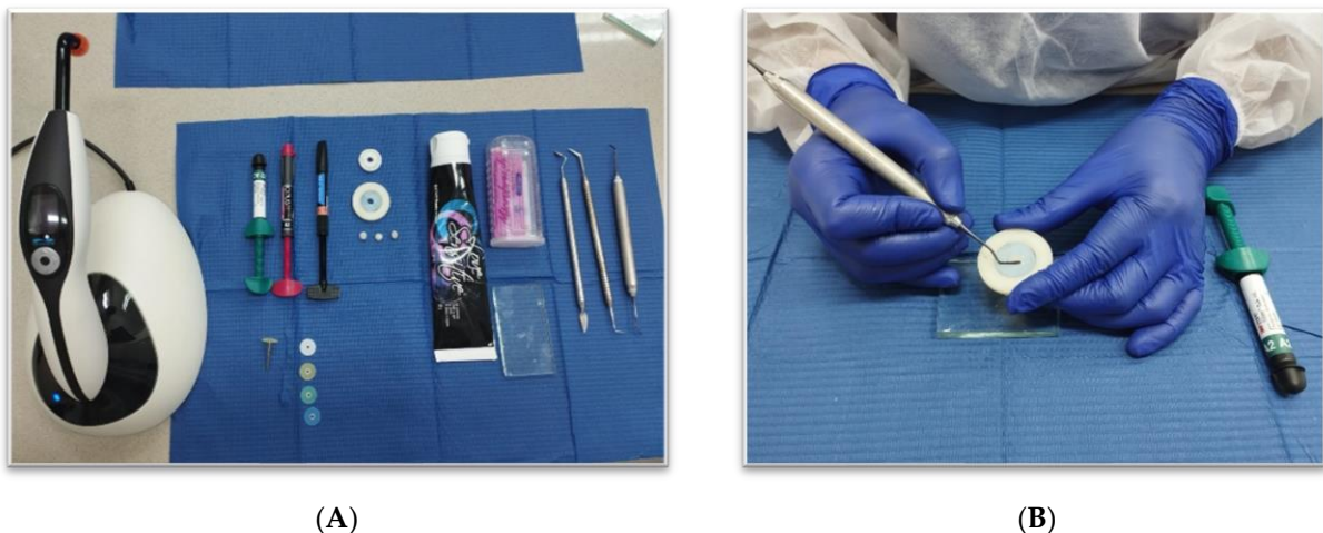
Figure 2. (A) Materials and instruments used; (B) resin composite compaction inside the block.
