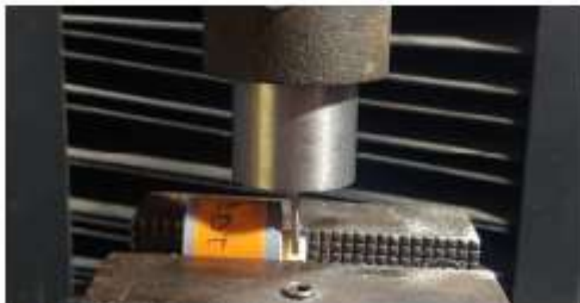
Figure 4. Shear test with universal testing machine.
