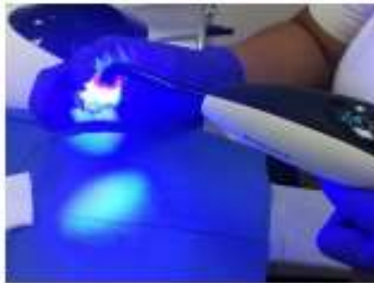
Figure 3. Light curing of Bulk-Fill resin blocks with LED unit.
